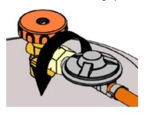
Place the quick-release regulator on the valve and press it down hard. If the switch is correctly turned off you will hear a characteristic click.
