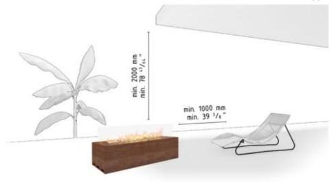
Figure 1: Minimum distance to flammable materials
