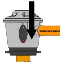
5. When the gas flow is required turn the valve of the bottle counter-clockwise.
