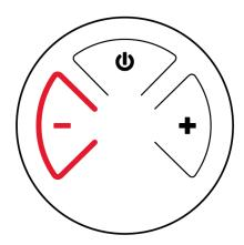
Press and hold "-" button to set appliance to pilot flame. Pilot flame remains burning (standby position).
