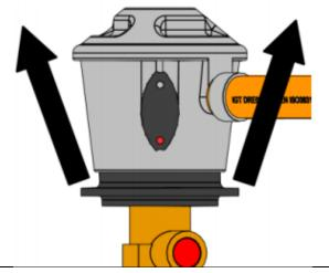
4. REPLACE the tightening cap on an empty or partially full bottle if it's not being used.
