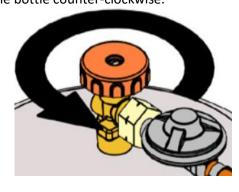
1. To let the gas flow in turn the switch into the ON position (or into the flame image).
