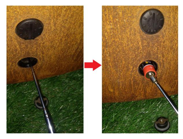
Photo 8: Removing the second battery from the container
