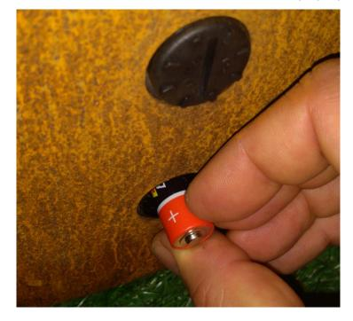
Photo 9: Placing the battery in the container
